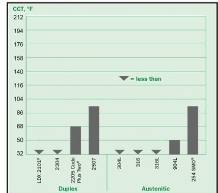
Critical Crevice Corrosion Temperature (CCT) in 10% FeCl<sub>3</sub>•6H<sub>2</sub>O
